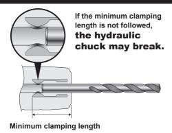
The minimum clamping length is marked on the hydraulic chuck.
