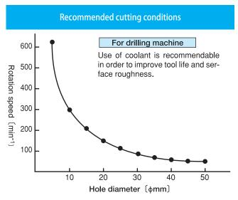
When using this insert with machining center, please adjust cutting speed between 40 and 100m/min.
