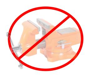
Don't use an ordinary vise to clamp your tool holder! Your tool holder may get damaged or deform the V-Flange and lose the accuracy.
