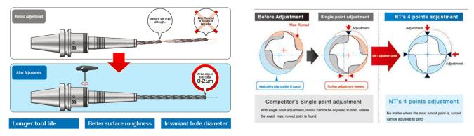
Zero runout is important especially when you are using a long drill. Like our 4D measurement, the further out you get along the cutting tool, the bigger the runout measurement is recorded. However with the R Zero, you will take runout to zero at the tip of the cutting tool. This will lead to invariant holes, better surface finish using ball end milling, long drill applications, and more. Online catalog
