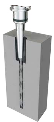
細穴奥の高精度穴加工 High precision cutting in a deep/narrow hole.
