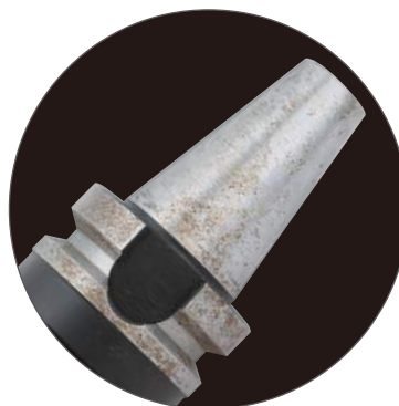
通常お社品サビ発生面 Rusted surface of standard product
