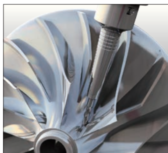
Finishing with ball endmill on 5-axis machine
