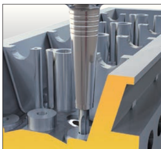
Reaming in tight space
