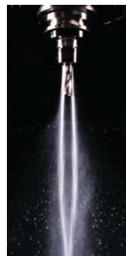
Cutter without oil hole FDC-C type R.P.M. .... 8 000rpm Coolant ..... 580psi Pressure
