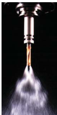
Cutter with oil hole FDC-OH type R.P.M. .... 8 000rpm Coolant ..... 580psi Pressure
