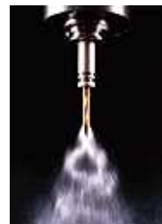
Cutter with oil hole FDC-OH type R.P.M. .... 8,000rpm Coolant ..... 870psi Pressure
